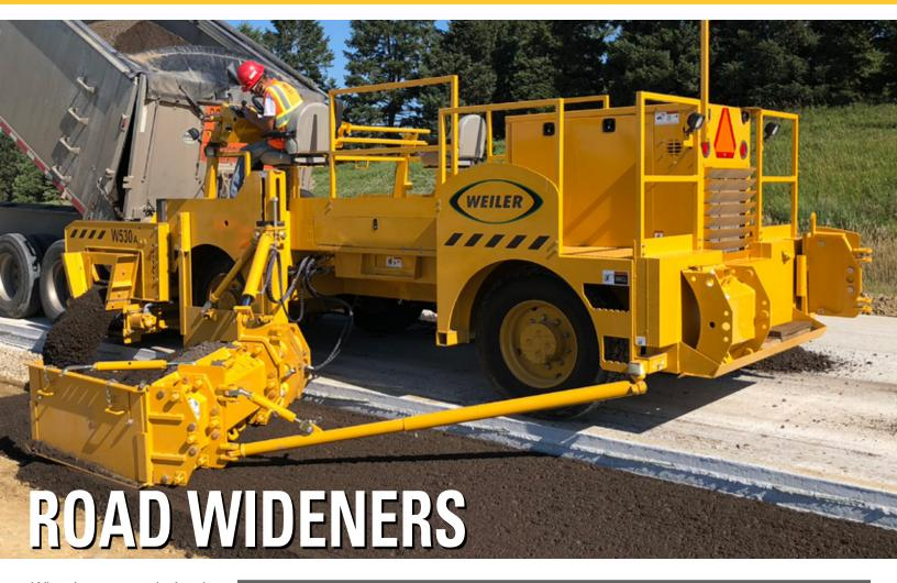
When it comes to placing the right amount of material at the correct grade and slope in one pass, whether on a shoulder or elsewhere, the best machine for the job is a Weiler road widener.
