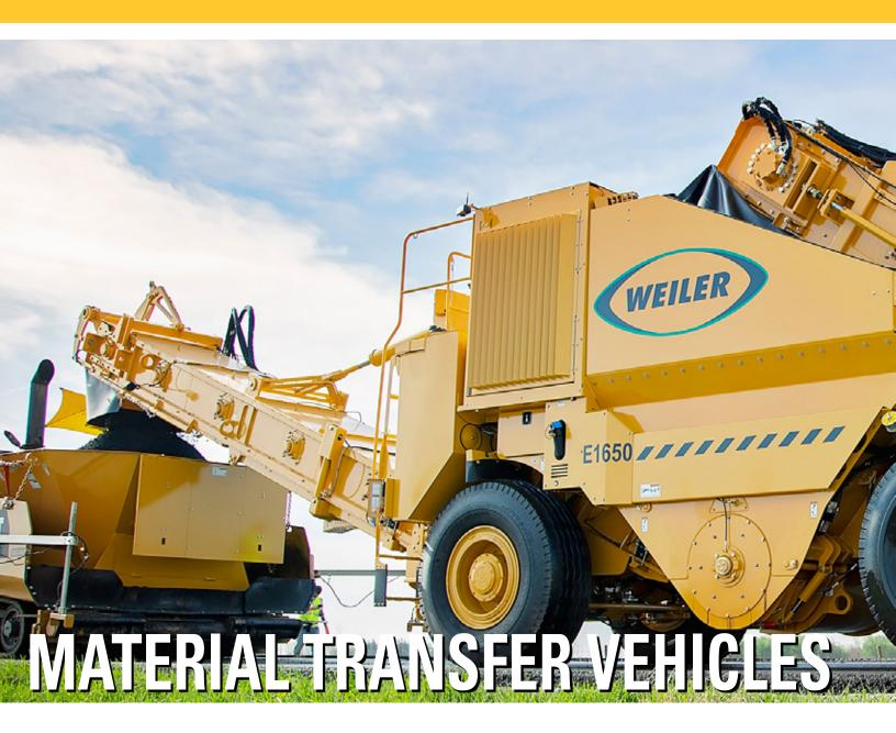
Material transfer vehicles provide nonstop, non-contact paving while reducing particulate and thermal segregation for smooth, long-lasting roadways.
