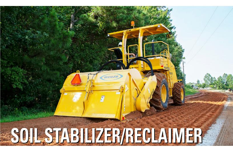
Engineered to perform in a variety of applications, the Weiler S200 Soil Stabilizer is available with two rotor options.
