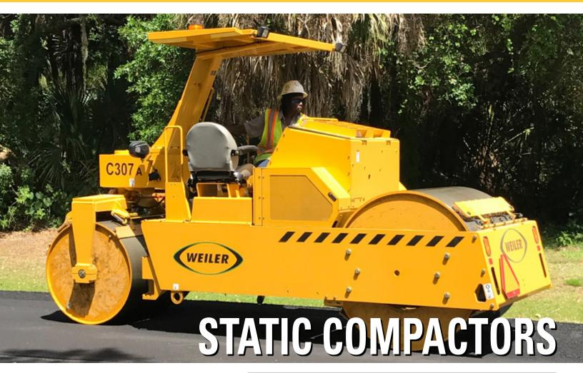
When static compaction is required, the Weiler 7 ton (6.35 mt) and 10 ton (9 mt) models perform in a wide range of applications from highway construction to driveways, base to finish layers. Linear force is easily adjusted by adding or reducing ballast in the drums.
