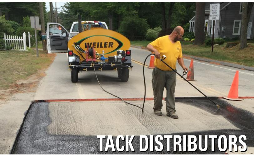
Weiler tack distributors are available in 250 gal (946 L) or 500 gal (1892 L) configurations. They are powered by a 5.5 hp (41 kW) Honda engine with clutched pump for easier starting and electric start option. The direct-drive pump is designed for asphalt with a capacity of 15 gpm (57L/min).
